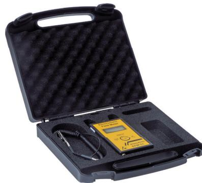
Handheld, portable, digital electrostatic field meter, detects and measures electrostatic fields.
